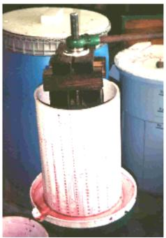
rotating the horizontal basket. Horizontal presses are simple and easy to operate, and they save wineries a tremendous amount of labor. The *Vaslin* presses were made with fiberglass baskets and
