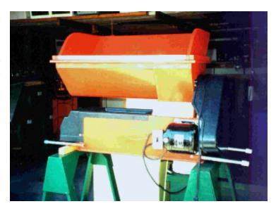
the hopper full of grapes. Power crushers save a great deal of labor, but they are expensive. Small power crushers made of painted steel sell for six or seven hundred dollars. The same machine fabricated from stainless steel, sells for about \$1000. Justifying the expense of a power crusher is difficult for home winemakers unless several barrels of wine are made each year.
