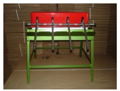
and six spout machines are common, but gravity bottle fillers as large as 24 spouts are produced. Two, three and four spout fillers are suitable for home winemakers producing 50 or more gallons of wine each year. Large gravity fillers are used by smaller commercial wineries. Many gravity type fillers will fill at a rate of about two bottles per spout per minute. One person is kept quite busy removing and replacing bottles.
